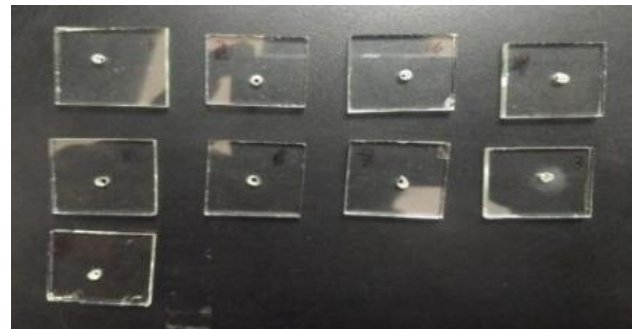
Figure.7: Holes machined by static USM
