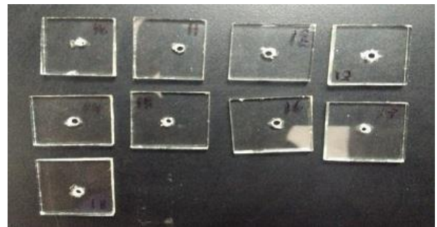
Figure.8: Holes machined by rotary USM at 500 rpm
