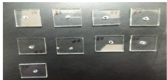
Figure.9: Holes machined by rotary USM at 1000 rpm
