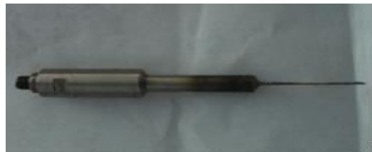
Figure.3: Horn with tool
