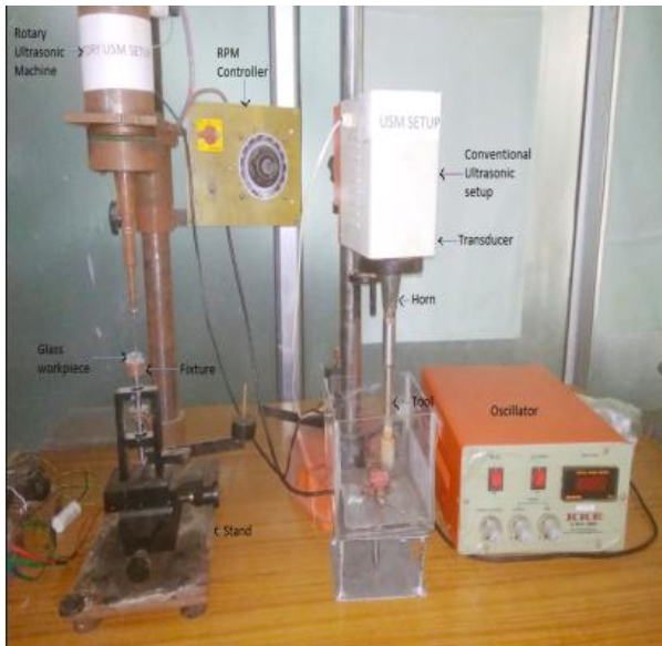
Figure.5: Setup of static & rotary ultrasonic machine
